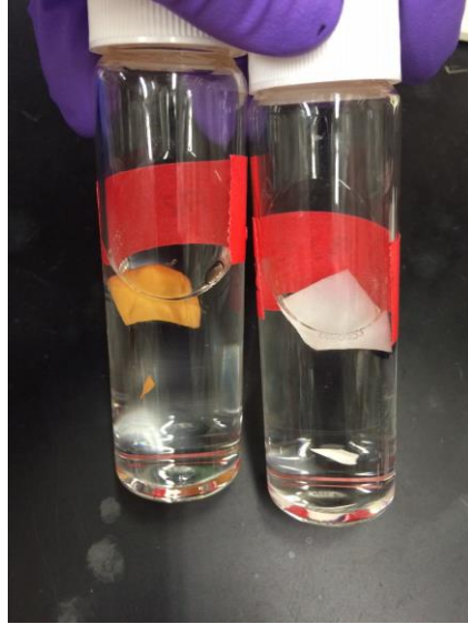
Figure 3.5. Representative images of Fh3 (at left) and Fh3-CTAB3 (at right) composites after digestion in 5 M H_2SO_4 for 24 h with constant mixing (0.125 g/L composite loading), indicating greater total solution phase availability of the iron oxide in ternary composites.
